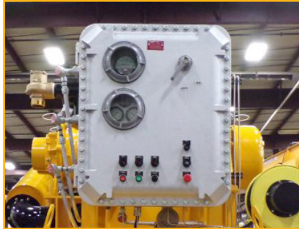
NEMA 7/9 CONTROL PANEL
